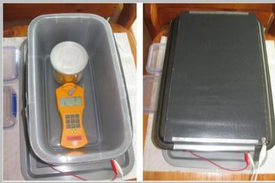
This is a photo of a basic built lead shielded test chamber, with a 15mm thickness of lead.
