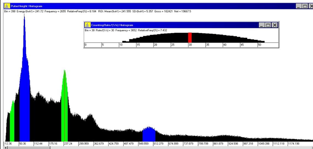
This will highlight the peak in a colour, and the PRA software will calculate the **Gross** counts in the chart heading. Divide the **Gross** count by the length of time of the test in seconds, to get the CPS (counts per second).
