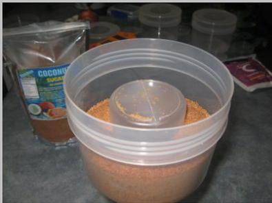
You need to have marinelli beakers to get the best test results, because this places the food or liquid sample for testing all around the scintillator crystal. This beaker design maximises the ability of your scintillator to detect radioactive contamination.
