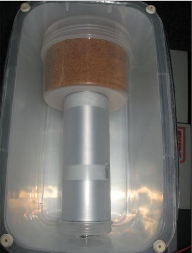
Here we have the Marinelli beaker full of coconut sugar, with the scintillator inside the test chamber.
